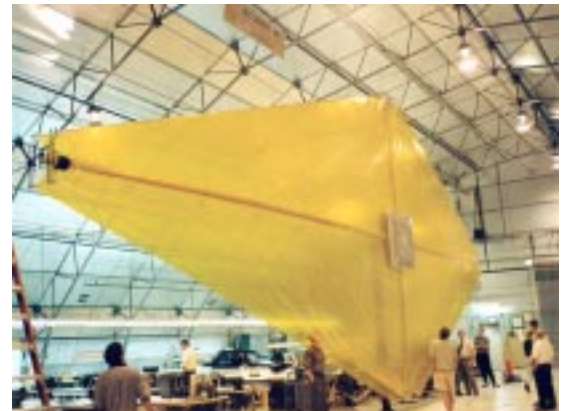
Figure 5.7: The Half-Scale Model of the NGST Sunshield.
