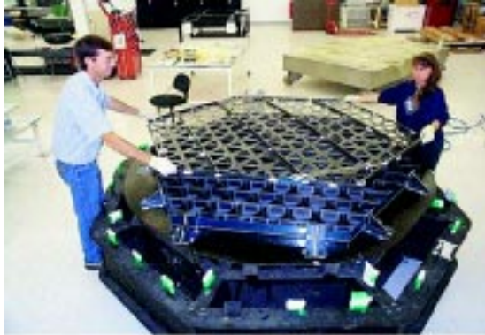
Figure 5.4: The University of Arizona Mirror System. A thin glass meniscus is mounted with a bed of active actuators to a stiff backing structure.
